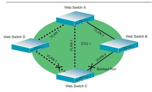
Figure 2-4 VLAN 3 Isolated in a Single Spanning Tree Group
